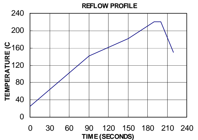
Figure 19 SMT Reflow Profile
